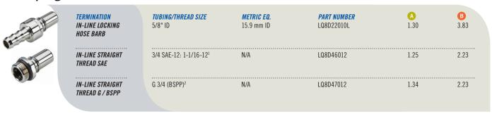
Note: <sup>1</sup>All SAE terminations are compatible with SAE J1926-1 ports. <sup>2</sup>All G (BSPP) terminations are compatible with ISO 1179-1 ports.
