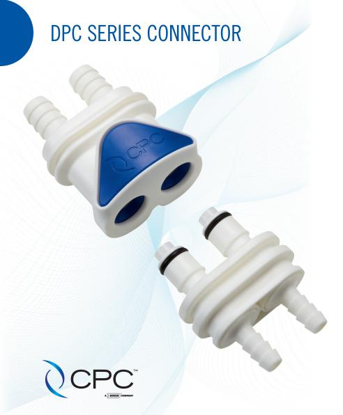
The 1/4" flow DPC Series couplings feature a dual port connection in a contoured design that delivers ease-of-use and excellent flow in a compact size. Made from acetal thermoplastic, the DPC Series includes valved and non-valved couplings with a single plastic thumb latch. One-hand operation makes the DPC Series the choice for simple, simultaneous connections and disconnections where two fluid lines are required.
